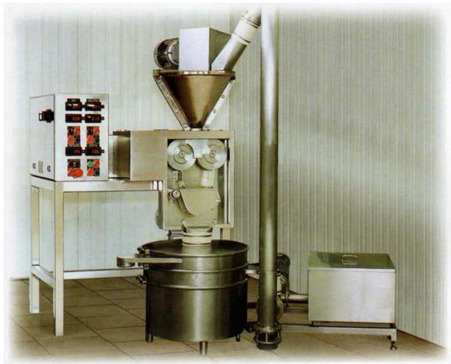
Small production units of briquettes or granules using these micro-compactors have also been designed and enable to obtain a briquettes or granules output of 50 kg/hour.
